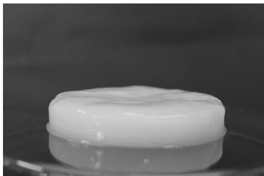
Fig. 2 Bacterial cellulose produced by a bacterium belonging to the genus Gluconacetobacter sp. Note that the appearance resembles a wet/damp leather
