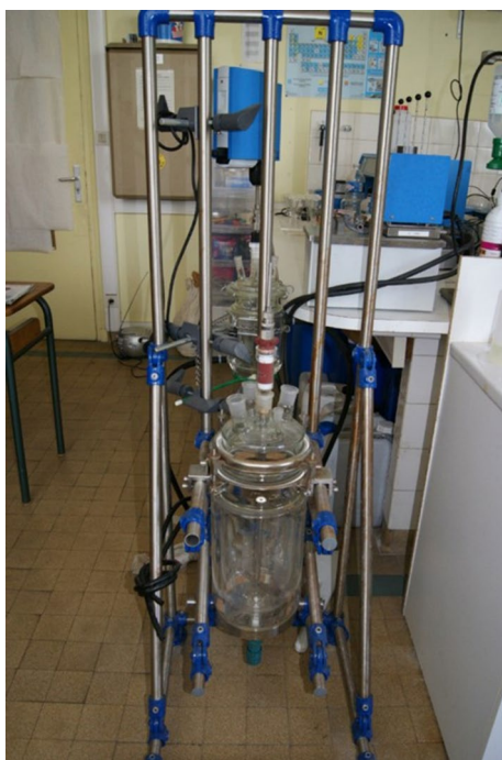
Fig. 3 Pilot used for the synthesis of cyclodextrin–epichlorohydrin polymers in our laboratory. This pilot permits to prepare up to 50 kg of materials in a single step
