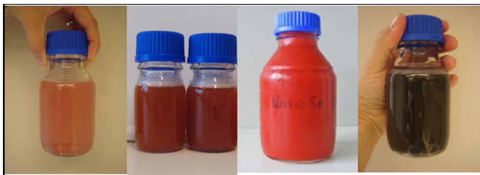
Fig. 1 Different possible colors of nano-selenium suspension after using of the biological synthesis method, where MRS medium, sodium hydrogen selenite, and bacteria strain were used (photo by El-Ramady, Nano Food Lab, Debrecen Uni., Hungary)
