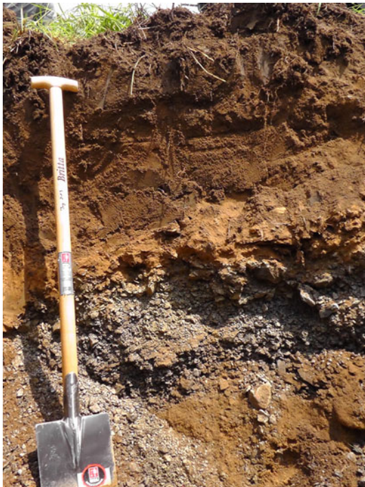
Fig. 2 Sediment/soil profile of a fluvial wetland sediment archive of the Main river (Germany). The profile shows distinct horizons and change in grain size and organic content
