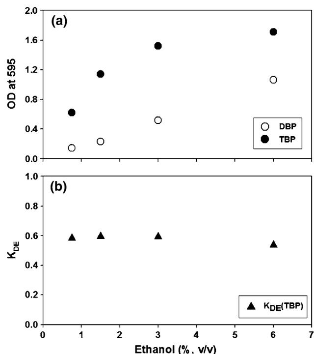
**Fig. 2** **a** Dichromate oxidation of ethanol-containing DBP and TBP. DR3 was used as the dichromate reagent, a microtube was used for solvent extraction and dichromate oxidation, and the times for extraction and oxidation were 1 h and 30 min, respectively. **b** Distribution coefficient for ethanol in TBP.  $K_{DE}$ (TBP) is defined as the ratio of the weight percent of ethanol in TBP to that in the aqueous phase. Autoclaved YPD media were used to prepare the standard ethanol sample
