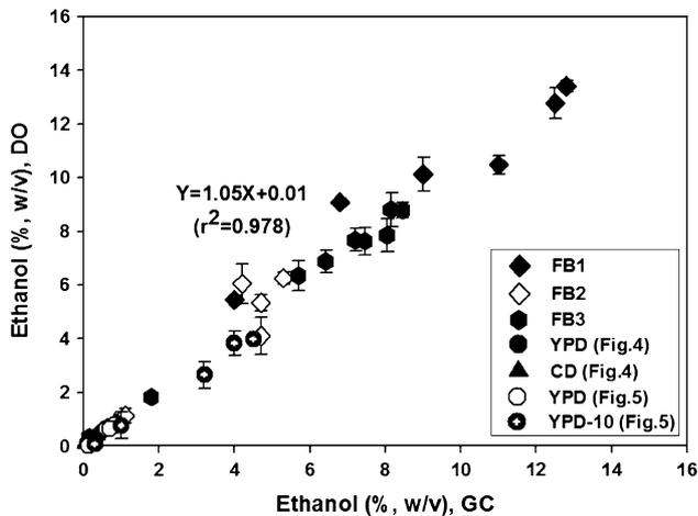
**Fig. 7** Correlation between the data from the two methods for measuring the ethanol concentration. Y-axis [ethanol (% v/v), DO] and X-axis [ethanol (% v/v), GC] were the data obtained from the solvent extraction-dichromate oxidation method and gas chromatography, respectively. FB1, FB2, and FB3 were the data ( $n = 3$ ) obtained from the fed-batch cultures in which the measurement was carried out in 96-deepwell microplate format
