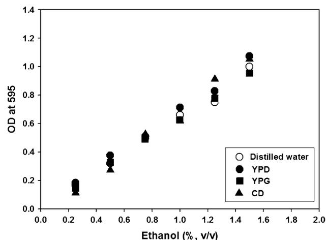
**Fig. 3** Standard curves for ethanol dissolved in distilled water, YPD, YPG and CD media. TBP and DR3 were used as the extraction solvent and dichromate reagent, respectively, a microtube was used for solvent extraction and dichromate oxidation, and the times for extraction and oxidation were 1 h and 30 min, respectively. Autoclaved media were used to prepare the standard ethanol sample
