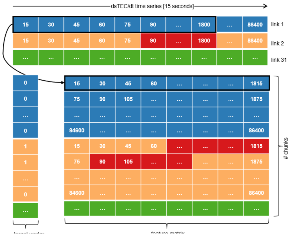
Fig. 3 Structure of the feature matrix related to the time values for DOY 259 (both for training and for testing). For every time value, the matrix is filled with the corresponding dsTEC/dt value. The red cells are an illustrative and hypothetical example to show the dsTEC/dt values perturbed from the earthquake and tsunami, corresponding to the value “1” in the target vector
