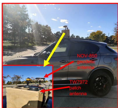
(a) Sensor box setup on the car roof
