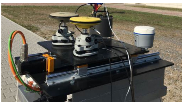
Fig. 1 Shake table and three GNSS antennas mounted on the table. The yellow antenna is Leica CGA60, which collects the observations for VADASE solutions, while the beige antenna is Novatel GPS-702, which collects the observations for RT-PPP solutions. The gray/white antenna is CHC I80, employed for the RP solution. The LVDT sensor is embedded under the black plate of the shake table
