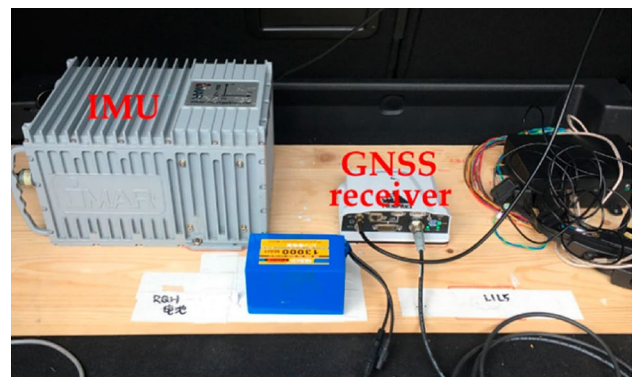
Fig. 5 Experimental layout for the iNAV-RQH reference system
