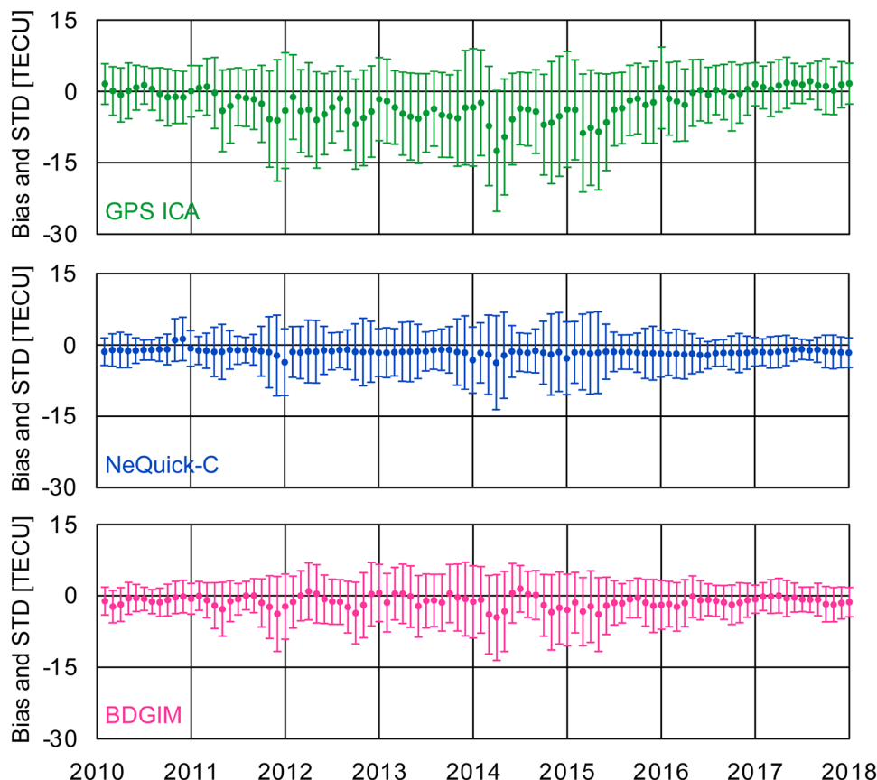
Fig. 4 Bias and STD series of GPS ICA (top)-, NeQuick-C (middle)- and BDGIM (bottom)-based VTEC estimates relative to the IGS-GIM during 2010–2017. Dots denote the mean difference between model-based and reference VTECs of each calendar month, and the length of vertical lines describes the respective standard deviations
