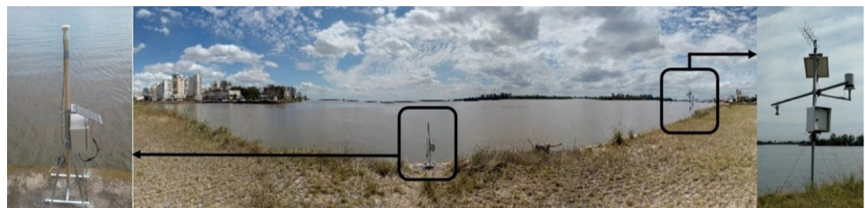
Fig. 1 GNSS-R sensor (left), experimental station site (middle) and radar gauge (right)
