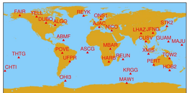
Fig. 16 Distribution of the selected IGS multi-GNSS stations supporting global RUP for real-time online GNSS processing services
