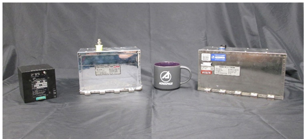
Fig. 1 Still life with space-qualified rubidium atomic clocks and an Aerospace Corporation-logged coffee cup. From left to right: Efratom/Rockwell GPS I, II and IIA atomic clock; PerkinElmer (now Excelitas) GPS IIR atomic clock; coffee cup; Excelitas GPS IIF atomic clock
