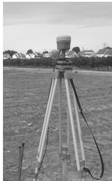
Fig. 1 Geodetic-quality GNSS antenna located in the experiment zone
