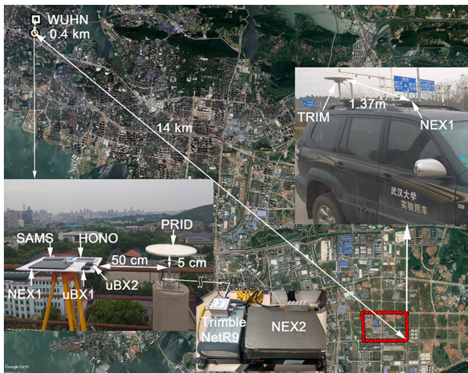
Fig. 1 Illustration of the distribution of all devices, stations and their antennas. The device and station configurations are listed in Table 1
