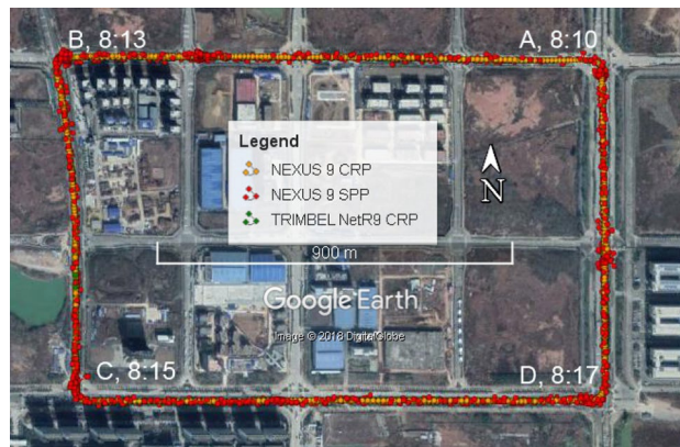
Fig. 13 Trajectory of the kinematic CRP solutions of TRIM (green line), NEX1 (yellow line) and the SPP solutions of NEX1 (red line) in suburban environments. The arrival time of the vehicle at the four corners is plotted
