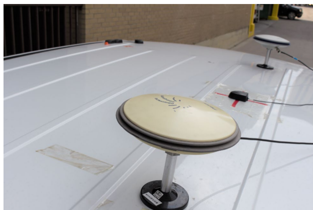
Fig. 12 NovAtel and patch antennas mounted on top of the land vehicle used in the field test
