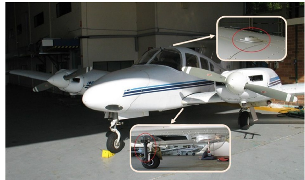
Fig. 4 Experiment aircraft and antenna setup. The GPS antenna is located on the top and the Locata antennas are on the underside of the aircraft
