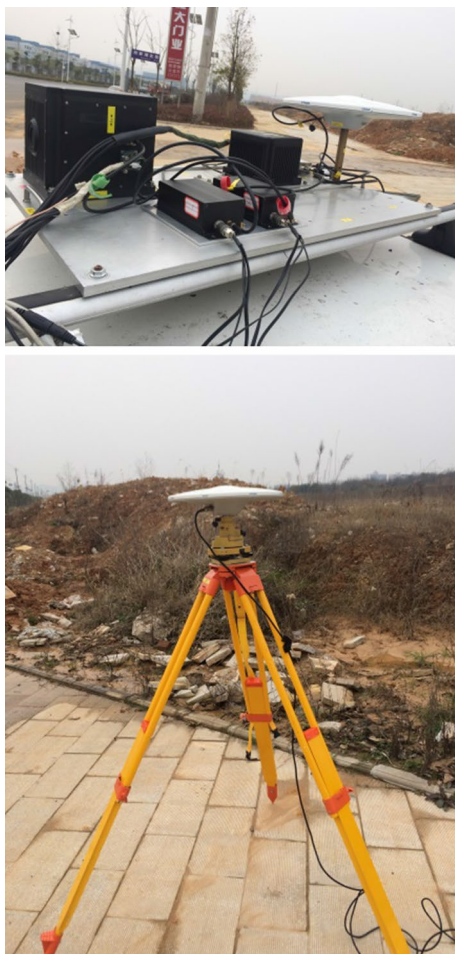
Fig. 2 Data acquisition equipment of rover (up) and base (bottom) in field test
