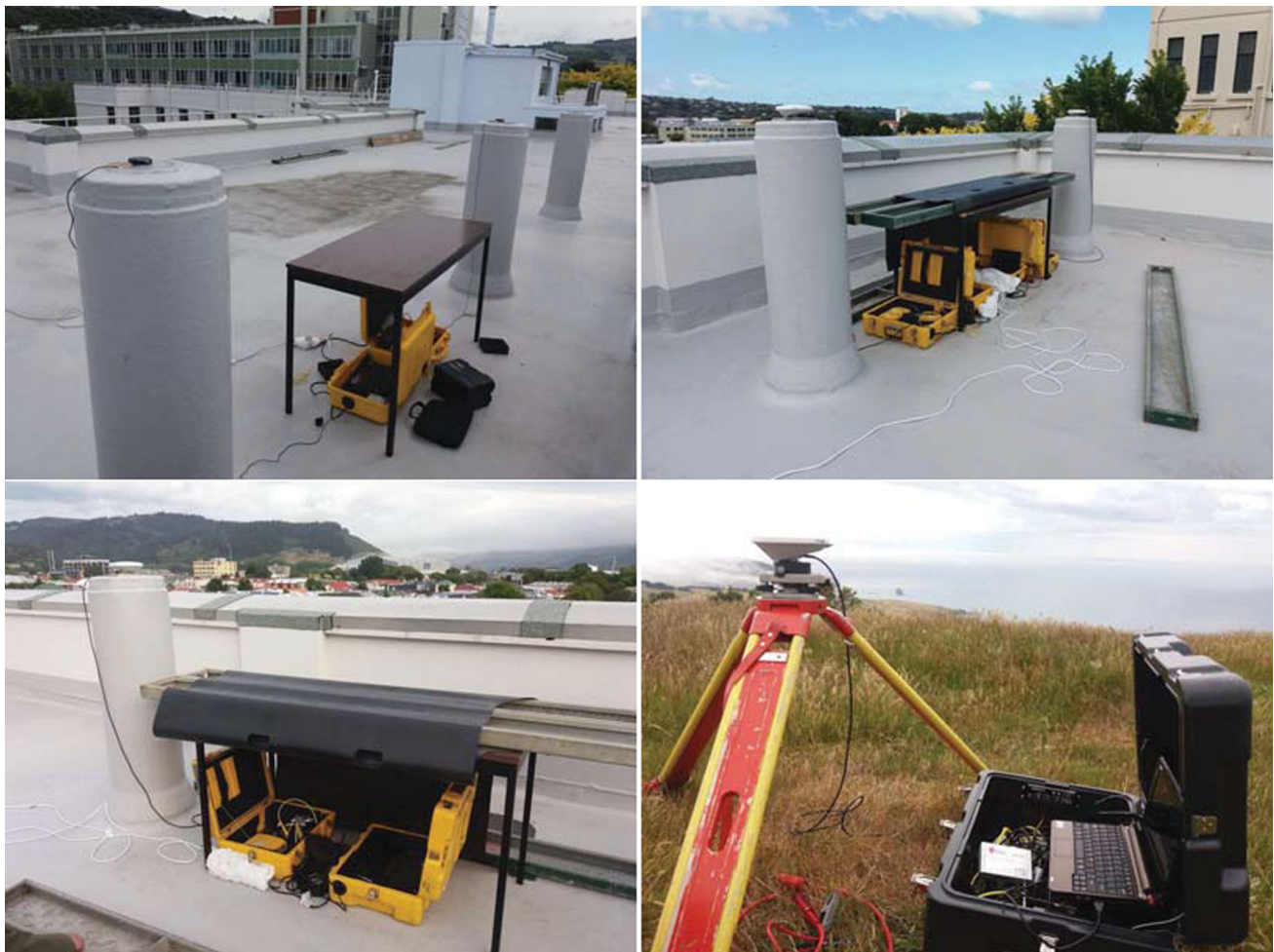
Fig. 1 GNSS ublox EVK-M8T receivers collecting data for GPS + BDS single-baseline RTK, with patch antennas ( top, left ) and Trimble Zephyr 2 antennas ( top, right ) in January 4–6 and January 6–8, 2016, respectively. Survey-grade Trimble NetRS dual-
