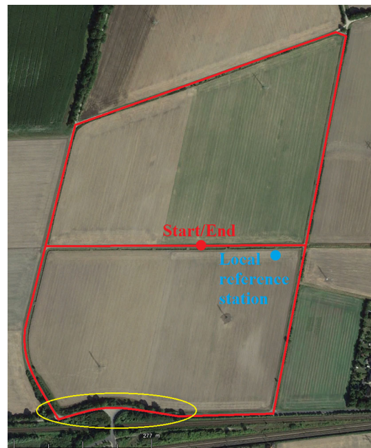
Fig. 2 Test track of about 500 \times 800 \text{ m} . The yellow ellipse marks an alley with signal obstructions
