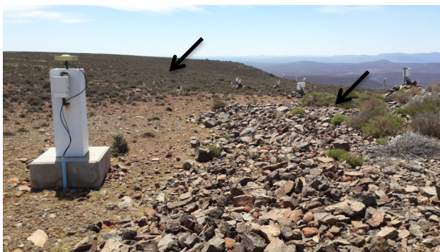
Fig. 1 Antenna of the GNSS station SUTM, Sutherland, South Africa. A cluster of 42 TDR sensors was installed 20–40 m northeast of the GNSS pillar ( white boxes in the background are the logger and multiplexer boxes of the TDR system, black arrows mark the border of the cluster). In the east and south the top surface consists of boulders from construction material, visible on the right side of the photo (photo provided by Chantal Fourier)
