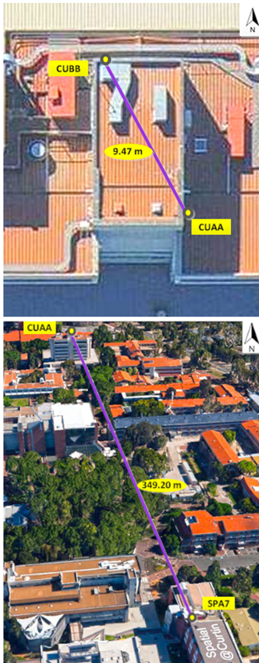
Fig. 1 IRNSS L5-enabled GNSS stations at Curtin University comprise of JAVAD TRE_G3TH_8 receivers connected to TRM 59800.00 SCIS antennas. Top CUA–CUBB. Bottom CUA–SPA7
