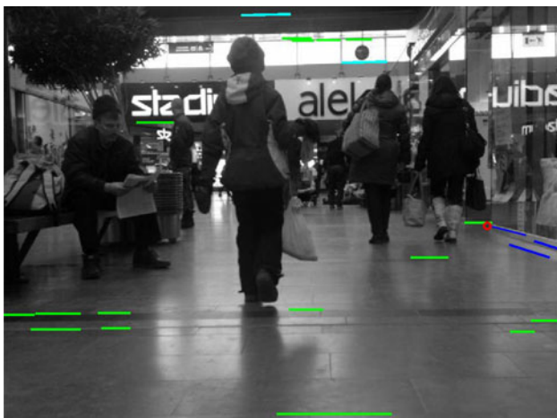
Fig. 2 Erroneous vanishing point location (shown with red dot ) due to poor line geometry
