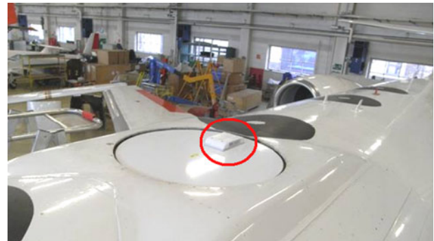
Fig. 19 ANASTASIA navigation antenna mounted on top of test aircraft
