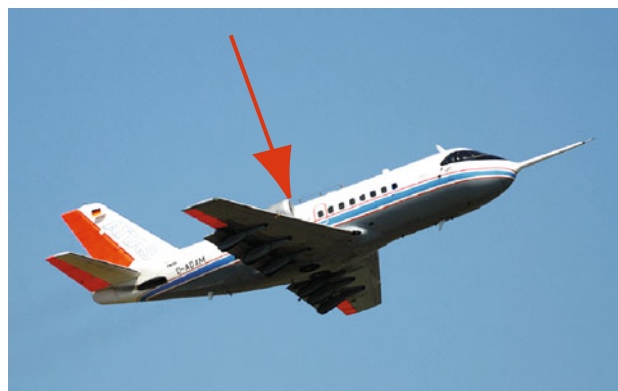
Fig. 1 The advanced technology aircraft testing system ATTAS in flight. The location of the GPS antenna is indicated by the red arrow
