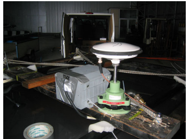
Fig. 3 The GPS/INS equipment and the van used to collect real data (INS is packaged in the box while round GPS antenna can be seen)
