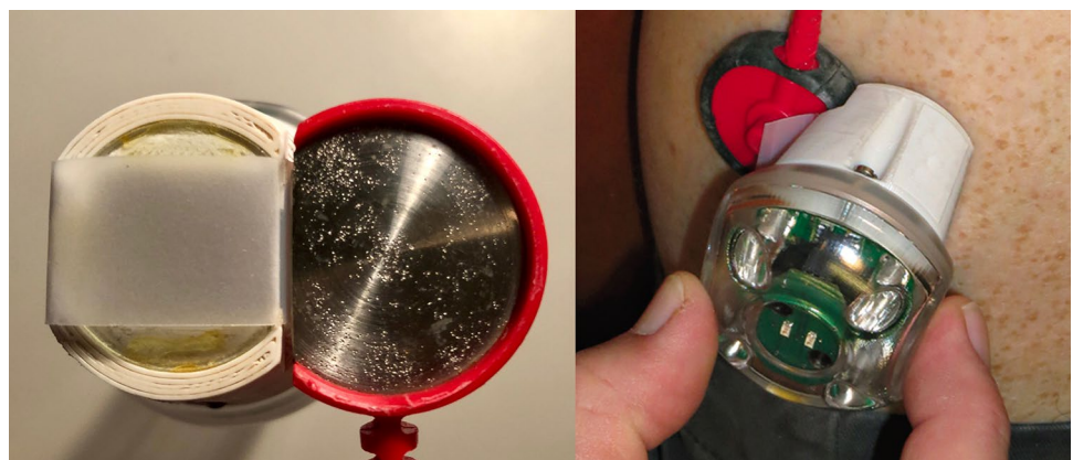
Fig. 1 The camera used in the sensitive sweat test is seen from below, adjacent to the D-shaped acetylcholine iontophoresis capsule, with starch tape stretched over the viewing screen (left) and in position to record axon reflex sweating at the medial calf (right)
