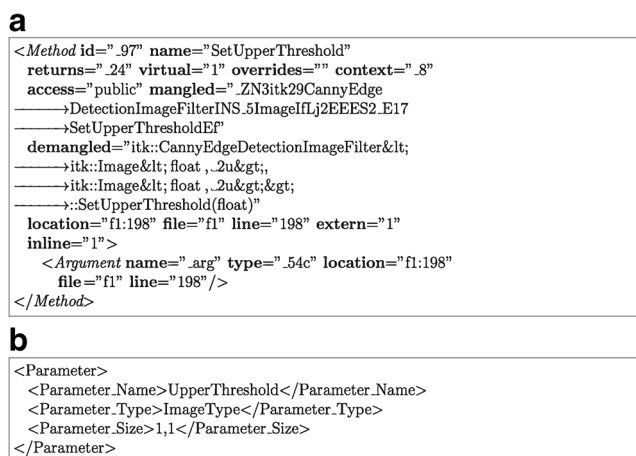
Fig. 3 A comparison of the XML files generated by WrapITK and what is ideal for SimITK. a Sample WrapITK XML. b Final SimWrapITK XML
