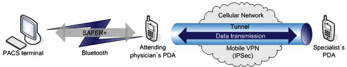
Fig 3. Secure wireless transmission of radiological image through Bluetooth with SAFER+ scheme and through CDMA 1×-EVDO with mobile VPN.
