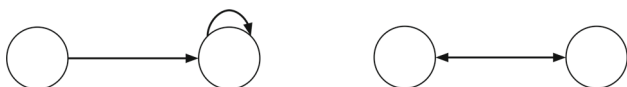
Fig. 1 Multiple instances of a transition system for the constraint: every state must reach a state that is reachable from itself
