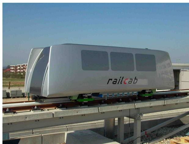
Fig. 1 RailCab prototype in scale 1:2.5 on the university test track
