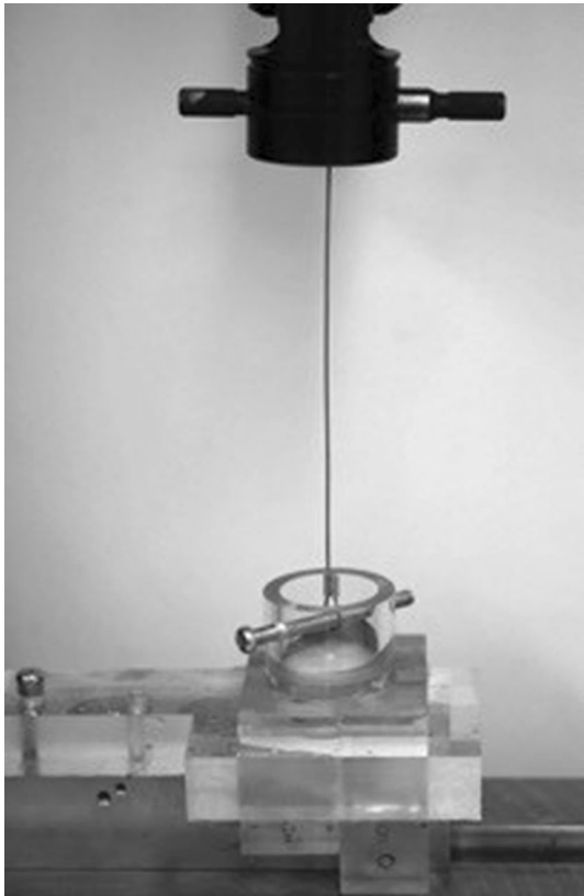
Fig. 2 Experimental tray fixed on an autograph
