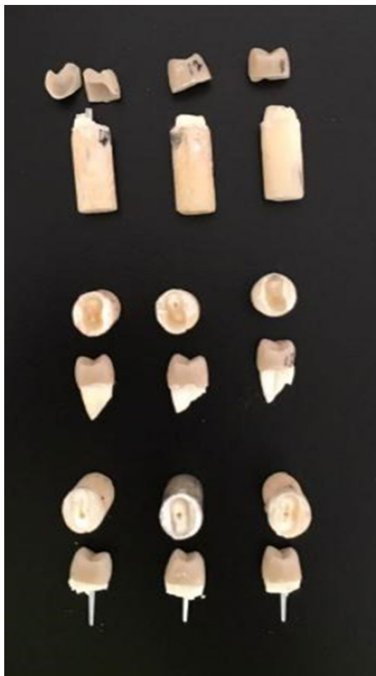
Fig. 3 Representative views of restorable (the first line) and unrestorable (the second and third lines) fracture modes
