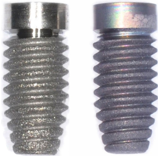
Fig. 1 The type of implants used in the study ( Left titanium, Right zirconium )
