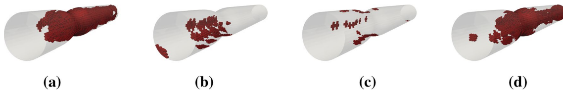
Fig. 5 Reduced mesh for NS operators of the HROM. The panels represent the cells of the full mesh (red elements) required for the calculation of the coefficients used to impose the interpolation constraints on DEIM. The background geometry refers to the mean geom-
