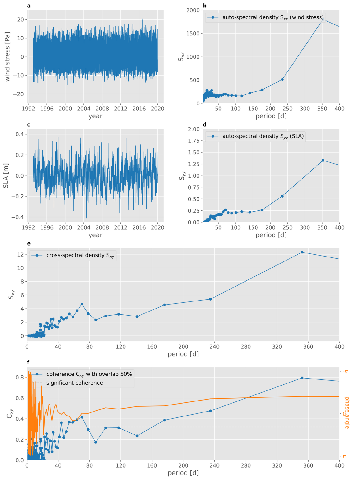
Fig. 1 Coherence at 55.75°W, 36.25°S. Time series of along-shore wind stress (a) and SLA (c). Auto-spectral density for a given time series of wind stress (b) and SLA (d). Cross-spectral density of both
