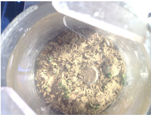
Fig. 2 Sediment surface of a core from Franks Tract, July 30, 2014. The surface was mostly covered with tubes built by a freshwater worm Manayunkia speciosa and some macroalgae. The core is in the 10-cm-diameter erosion microcosm, and the 1.91-cm-diameter gray plastic disk in the center is to prevent erosion where shear stress is known to be greater than elsewhere during the experiment
