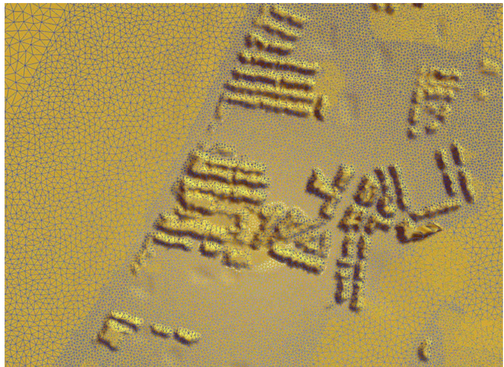
Fig. 6 Section of the mesh used by ANUGA to simulate the tsunami inundation. The finest mesh resolution is approximately 6 m between nodes which is sufficient to resolve individual buildings affecting the flows
