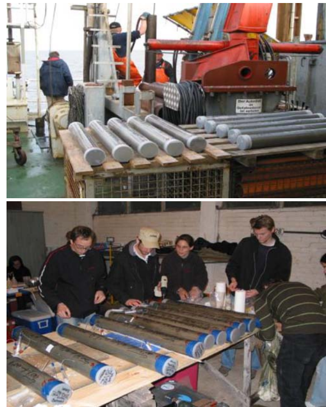
Fig. 7 Vibro-coring tidal flat sediments down to 6 m depth with an aluminium tube and recovery using a tripod
