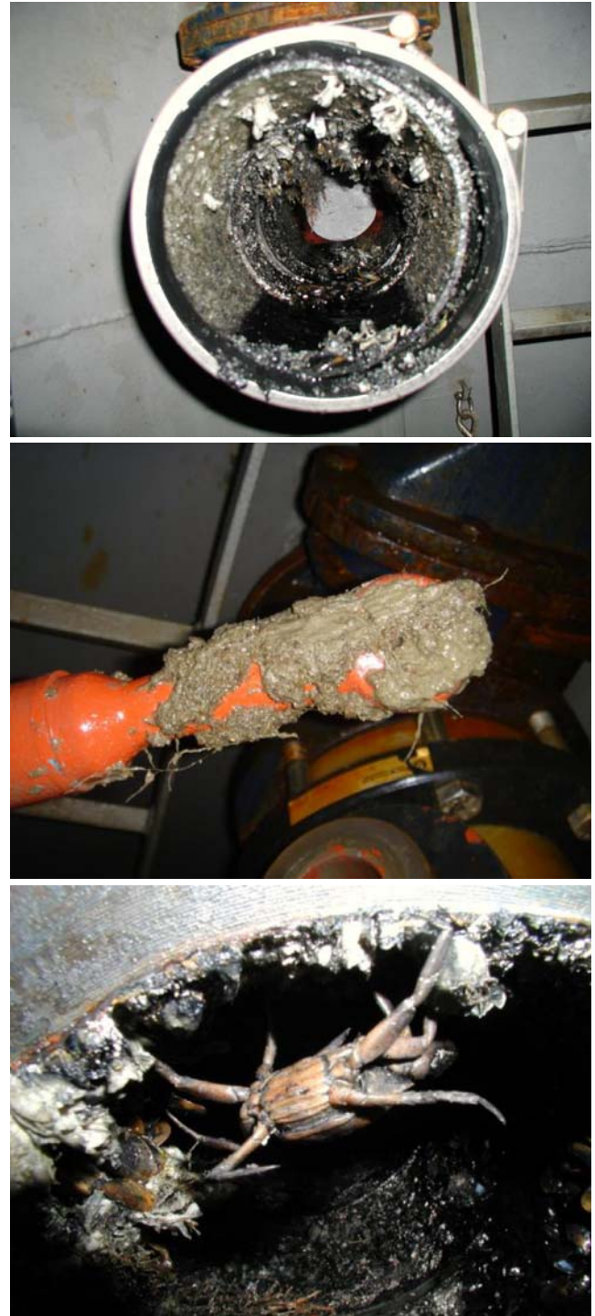
Fig. 3 Bio-fouling in the flow-through tubes of the time-series station and on a sensor recovered from one of the tubes
