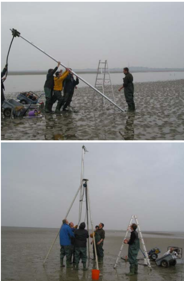
Fig. 7 Vibro-coring tidal flat sediments down to 6 m depth with an aluminium tube and recovery using a tripod
