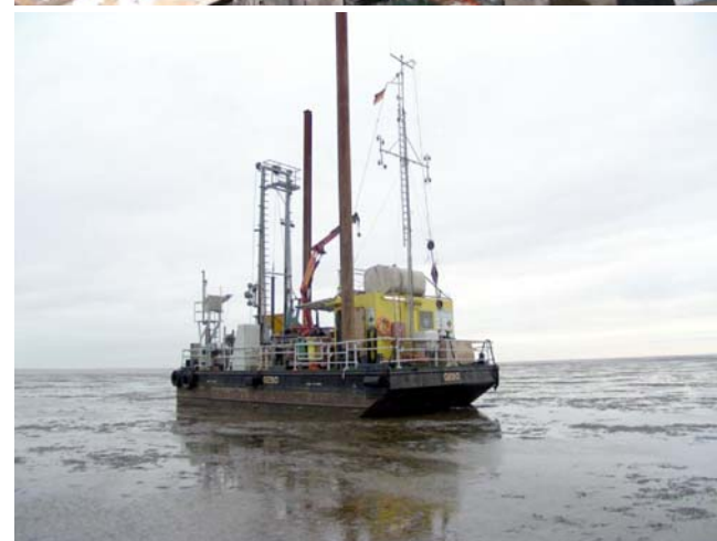
Fig. 8 The deep subsurface of the tidal flats (≈20 m, Holocene plus top of Pleistocene) was accessible with the help of a commercial drill ship
