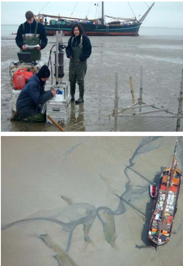
Fig. 9 A flat-bottom ship ( bottom ) was chartered for microbiological work on the tidal flats over 1–2 weeks using landers ( top ) to automatically measure the microbial activity in the surface sediments at high and low tide
