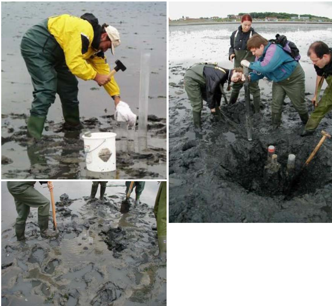
Fig. 6 Short sediment cores were obtained by driving plastic tubes into the sediment and digging them out afterwards
