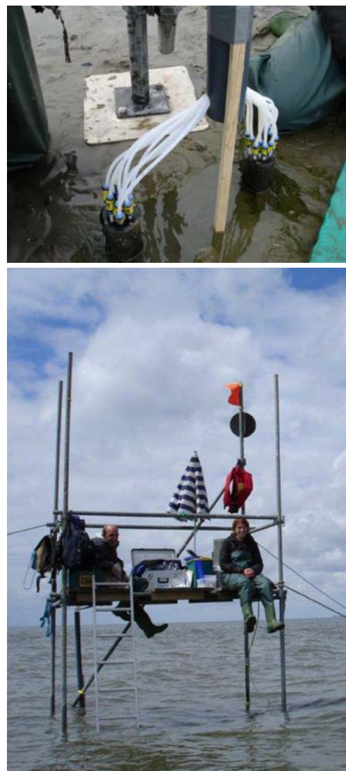
Fig. 5 Multiple outlets of the newly developed pore water sampler (top) and sampling at high tide (bottom; in good weather conditions only)
