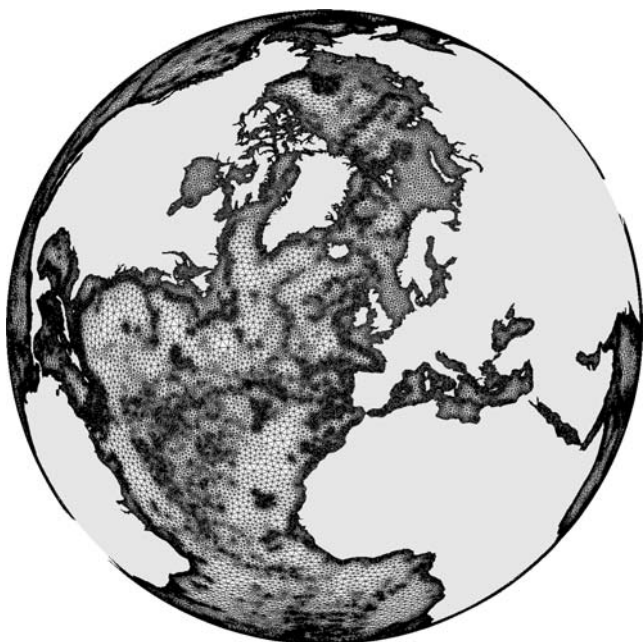
Fig. 9 Mesh of the World Ocean. The mesh size field is defined using a shore proximity function, the bathymetry, and its Hessian
