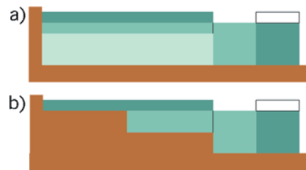
Fig. 3a, b Schematic representation of the bay-inlet system. a The bay has vertical side walls. b The area of the bay is a linear function of depth (see Maas 1997). The different colours focus on the fact that in a equal transport in the inlet (equal amount of subsequent entering packets of fluid) induces equal vertical displacement. The displacement in b decreases with the increase in the sea-level because the bay area is a function of the sea-level position. In this case more water through the inlet is needed to maintain equal sea-level rise, which indicates that the bay response is non-linear. The contouring lines above the second packet of fluid illustrate the fact that the packet can be displaced into the coastal area only if the water level is at least as high as the level in the bay. However, our simplifications do not consider this effect
