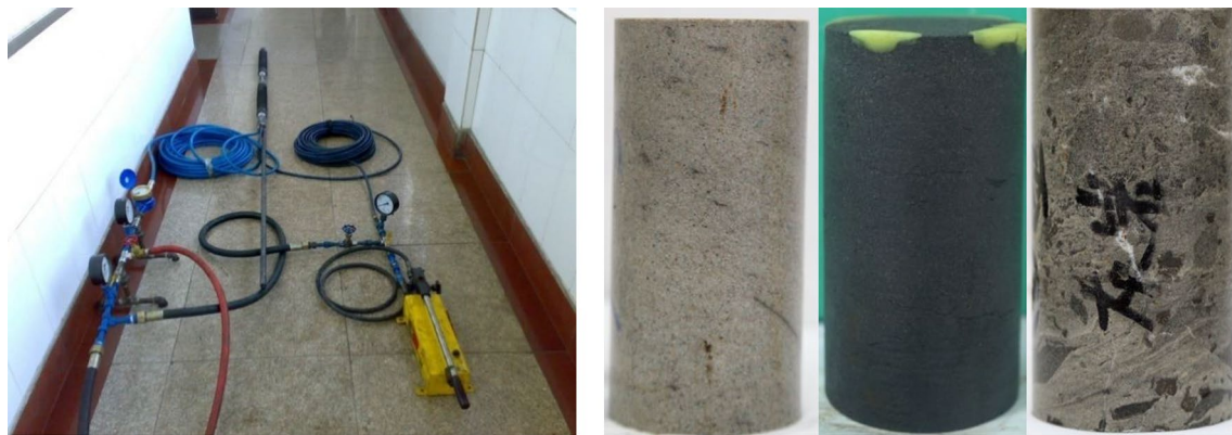
Fig. 3 Device of Packer test device and rock specimen photographs for the sandstone, mudstone, and limestone
