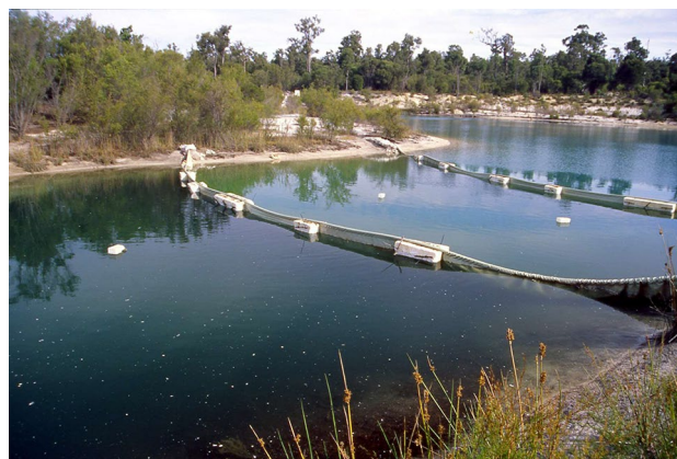
Fig. 4 Manipulative experimental macrocosms formed by sectioning of a pit lake arm by watertight curtains (Lund et al. 2006)
