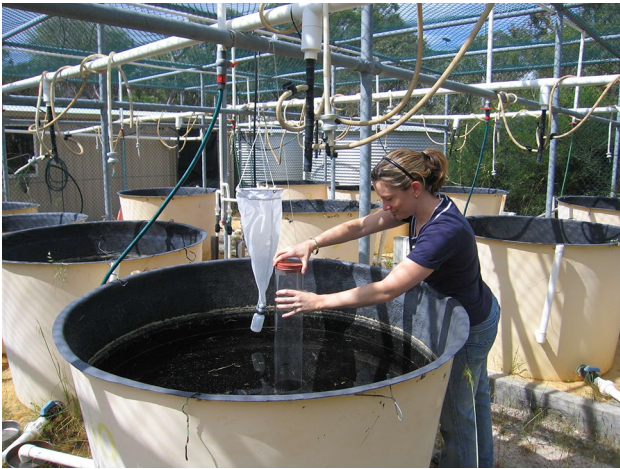
Fig. 3 Manipulative experimental mesocosms: 12 fibreglass 2000 L enclosures (Lund and McCullough 2009)
