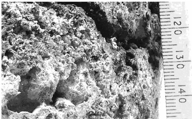
**Figure 2.** Reactive mixture after clogging
