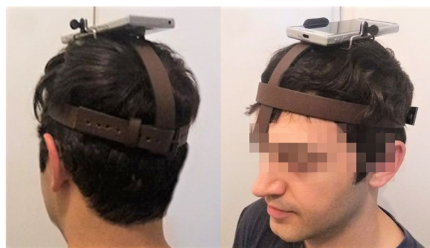
Fig. 4 The placement of the smartphone on the user's head for HeadGyro software switch
