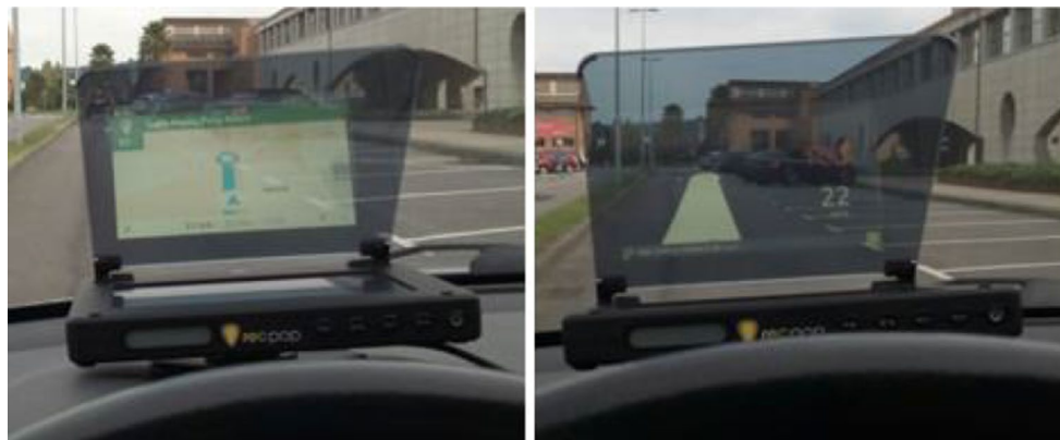
Fig. 7 Google Maps (left) and HUDWAY (right) applications running in the HUD device
