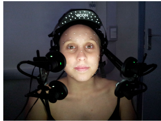
Fig. 4 Head-mounted MoCap system to capture facial expressions which have semantic meaning in Libras
