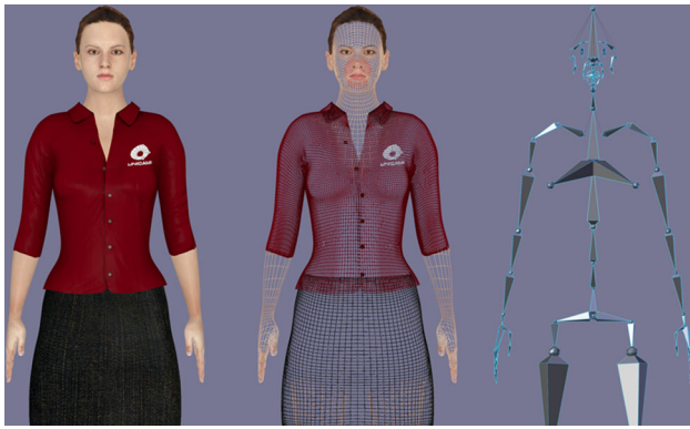
Fig. 8 The three-dimensional model of the avatar (from left to right): as presented to the user; polygon mesh; and control skeleton
