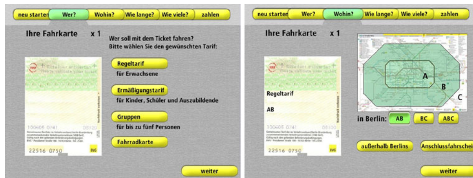
Fig. 2 Screenshots of the redesigned ticket vending machine applying inclusive design principles. Left : At the beginning of the process, the ticket is incomplete, and the users start with selecting who (or what) is travelling (a regular adult, a child, a group, or a bicycle).
