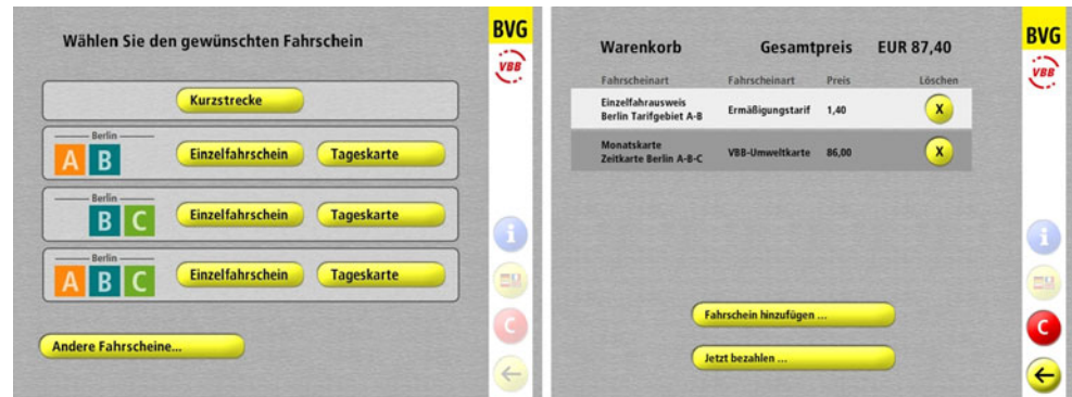
Fig. 1 Screenshots of the original version of the ticket vending machine. The left panel shows a screen for the selection of tickets for different tariff zones (short trip and zones AB, BC, ABC). The right panel shows the contents of the electronic shopping basket
