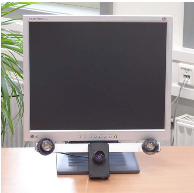
Fig. 9 Remote eye tracker system setup. The eye tracking hardware consists of a single high-resolution camera below the display and two infrared LEDs to either side
