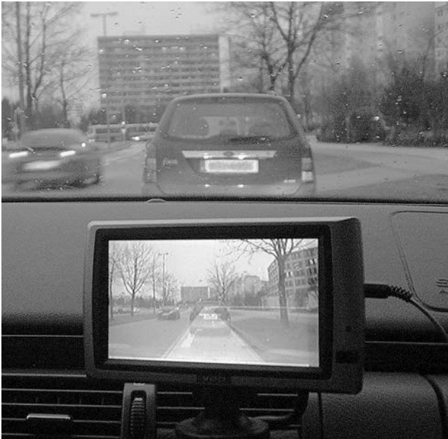
Fig. 17 AR car navigation prototype
